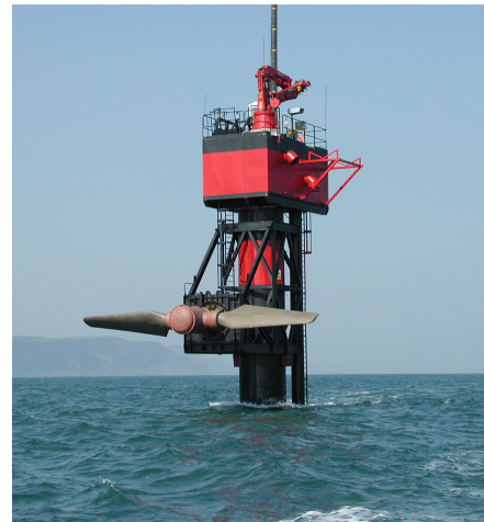
Figure 3: The Seaflow with the collar raised above sea level (used with permission).
